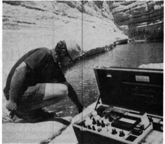
An investigator measures the salinity of springs in the Negev Desert. Irrigation using brackish desert aquifers is an Israeli specialty. "The shortage of water is one of the most limiting factors in economic and population development in Israel and in the Territories."
