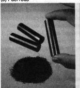
Both the thorium and uranium particles are mixed with a graphite material and formed into fuel rods that are 0.5 inch in diameter and 2 inches long.
