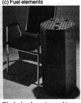
The fuel rods are inserted into holes that are drilled into the hexagonal graphite fuel element blocks, which are 14 inches in diameter and 31 inches long.
