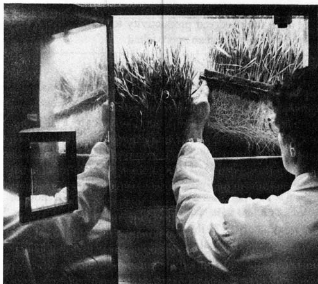
One of the growing chambers for the experiment described by Salisbury. His co-researcher, Dr. Bruce Bugbee, here lifts up the rock wool base of the plant-support system to show the dense root system of the 18-day-old plants. The inside walls of the chamber have mirror surfaces to maximize reflection of light, and at left is the reflection in the open door of the growing chamber.
