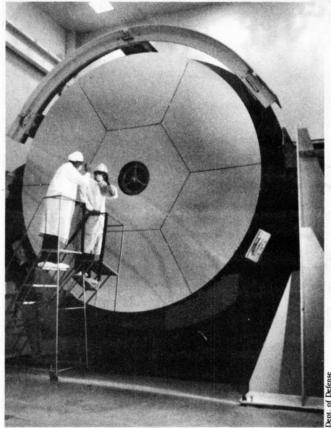
The LAMP mirror is an adaptive, segmented mirror currently in final stages of acceptance testing by ITEK Corporation of Lexington, Massachusetts. Here a technician checks the mirror surface after the seventh and final segment is in place on the supporting backplate. The extremely precise figure (shape) and alignment of the mirror's lightweight facesheets are controlled by actuators attached to the rear surfaces. The overall diameter of the fully assembled mirror is four meters.
