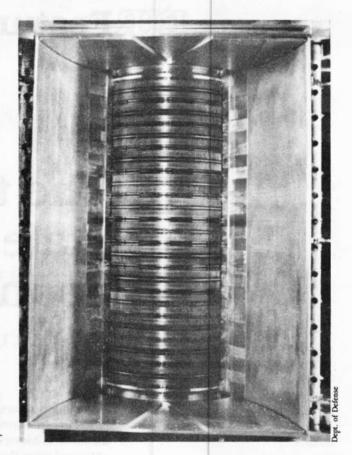
The cylindrical gain generator of the Alpha chemical laser is prepared for installation and testing at TRW's Capistrano Test Site. Alpha uses atomic fluorine and hydrogen to form the hydrogen fluoride lasing medium. The device then uses cylindrical mirrors to extract a 2.7 micrometer wavelength high-power laser beam. Alpha is the key component in the concept design for the SDIO's Zenith Star experiment.
