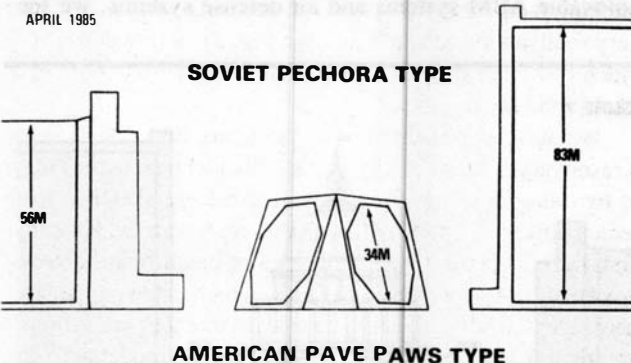
This DoD diagram compares the scale of the U.S. PAVE PAWS early warning radar located in Alaska with the scale of the existing Soviet ABM radar at Pechora and the new Krasnoyarsk ABM radar. Note that the Pechora measures 56 meters across its face, while the Krasnoyarsk measures 83 meters and the U.S. PAVE PAWS 34 meters.
