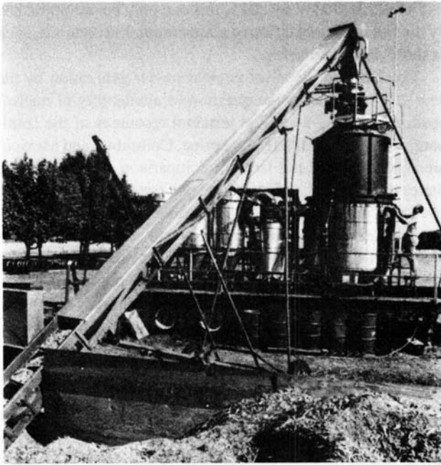
A gas producing unit utilizing "biomass"—a very low energy flux-density source—to turn farm products into fuel. In Brazil, vast amounts of food crops are wasted to produce such "self-sufficient" fuel, under the pressures of IMF financial policies.
