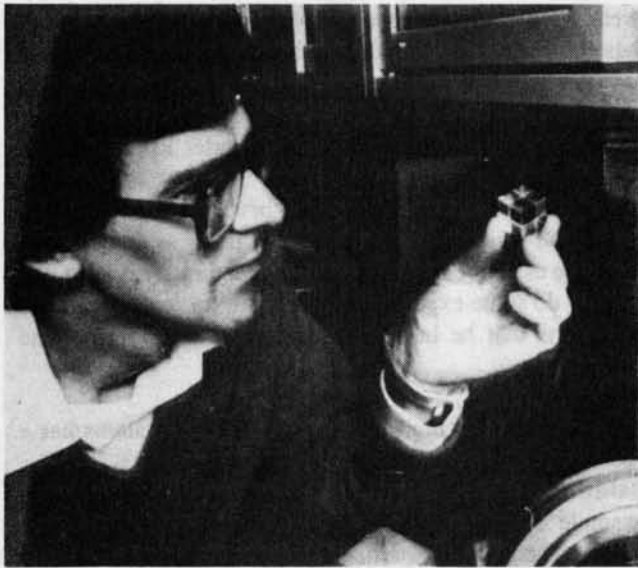
Graser crystals: The harmonic properties of crystals are currently utilized to transform the frequencies of electromagnetic radiation in the optical spectrum. For grasers, both the generation and propagation of the output, coherent gamma ray pulse will strongly depend on these crystalline harmonic properties. Shown above is Dr. Stephen Craxton, who demonstrated that KDP crystals could frequency-triple infrared light into light at ultraviolet wavelengths.
