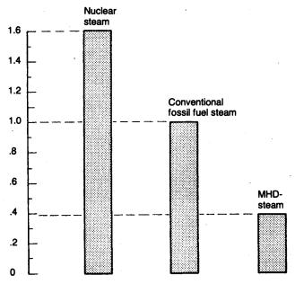
Cooling water requirements for power plants have generally dictated that they be sited on rivers, bays, lakes, or other large bodies of water. The two- to four-fold decrease in cooling water requirements for MHD systems means they could be sited more flexibly, where water would otherwise be a constraint in power plant construction.
