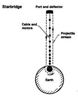
The Starbridge elevator connects a massive, orbiting space port and deflector with the surface of the earth. Counter streaming projectiles provide local support to the cable and motor structure.
