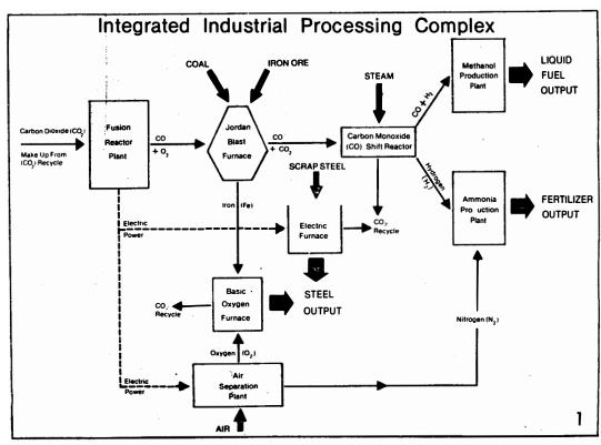
producing 2,000 tons a day of oxygen, will have to accompany each set of two blast furnaces converted.
