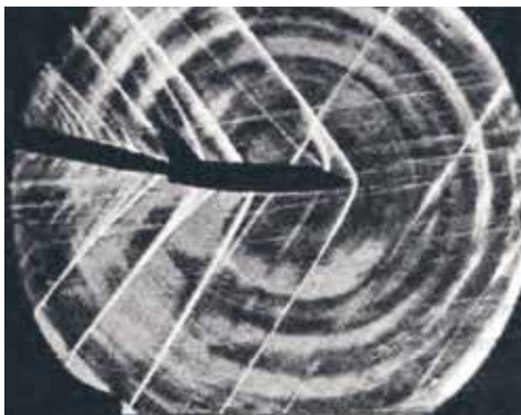
(b) Formation of sonic boom shock wave
