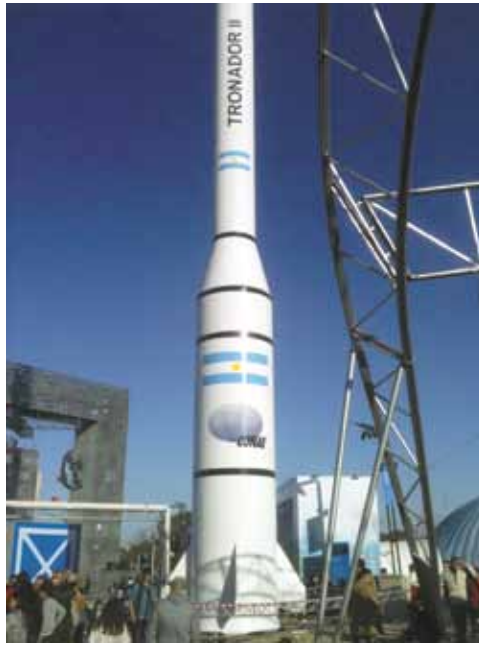
A mockup of Argentina's Tronador (Thunderer) II, a liquid-fueled rocket designed to lift payloads into Low Earth Orbit.
