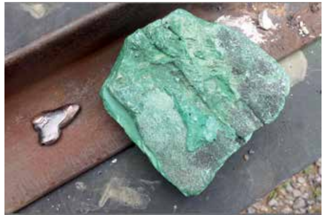
Thanks to charcoal, the copper on the left could be made from malachite, on the right.
