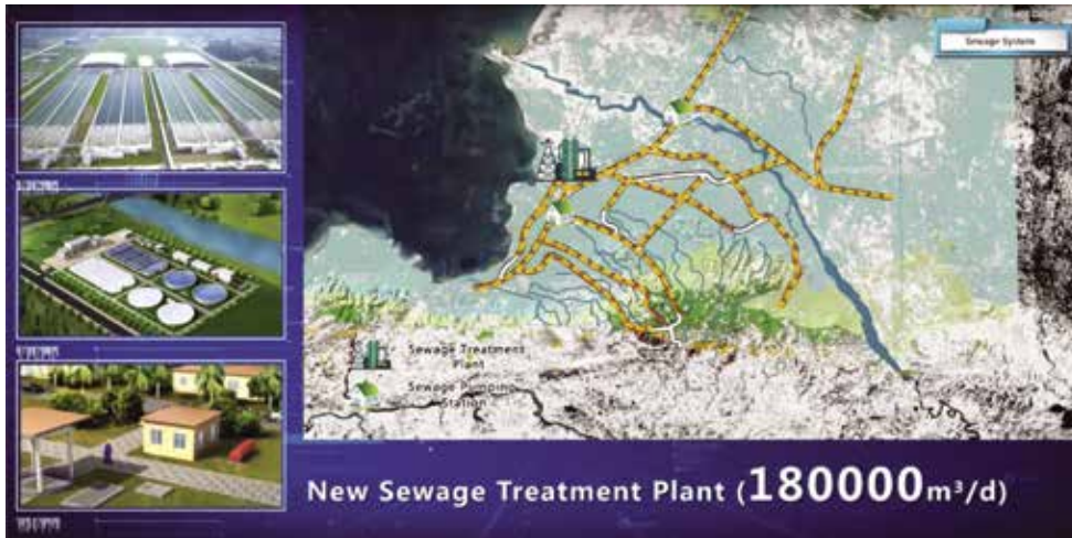
A sewage removal and treatment proposal from 2017—one component of a new, comprehensive infrastructure plan developed by China’s Southwest Municipal Engineering Design and Research Institute to renovate and rebuild Port-au-Prince and its port.
