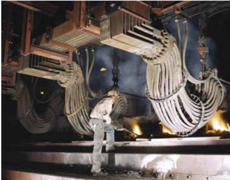
Industrial use of electricity per person is about 17 times that of residential. Shown here is a large electric phosphate smelting furnace at a TVA chemical plant the Muscle Shoals area of Alabama in June 1942.
